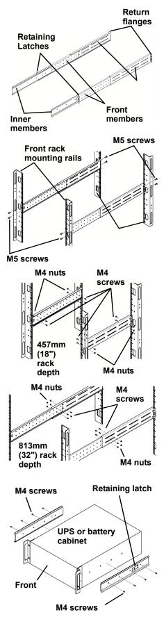
6. If available, apply a bead of grease 25mm (1") long at four (4) places inside the bottom, curved tracks of the front members as shown below right. The grease will allow the equipment to slide into the bracket assemblies more easily.
